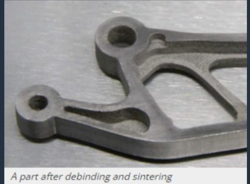
A part after debinding and sintering
