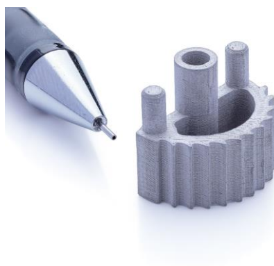
Fig. 1: Sintered engineering ratchet printed with CMG Tech-X 17-4PH HMs filament for use in bicycle shifter.
